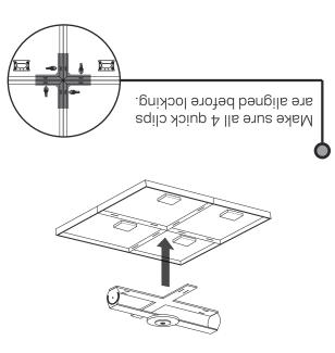
Place mounting bracket in center and align quick clip holes.
